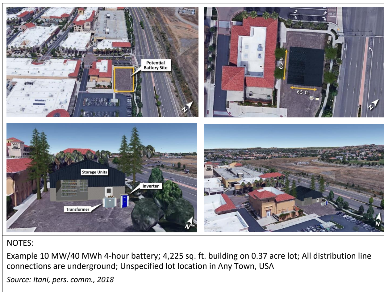
Figure 3-1513. Example Energy Storage Facility Enclosed in Building
